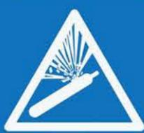
Only use containers designed for cryogenic service. As the liquid warms and turns into gas, the pressure rises, and containers that are not equipped with venting devices can catastrophically rupture.
